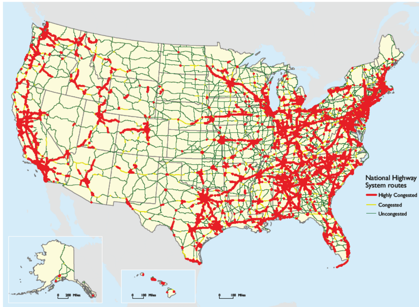
Figure 4-3 Peak-Period Congestion on the National Highway System: 2040
