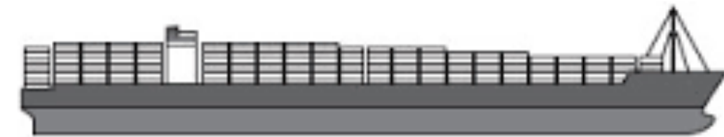
Panamax: max. load 5000 containers
